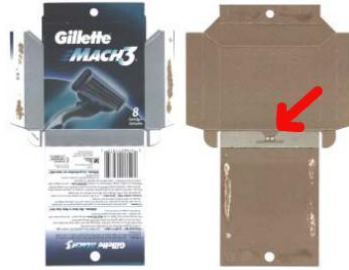
Fig. 11. Gillette pack with hidden RFID tag
