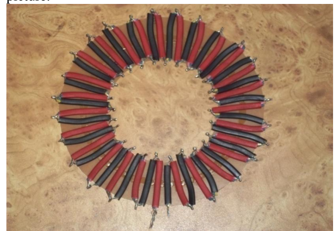
Fig 7 Completely fabricated thermopile mounted on the hollow GPB
