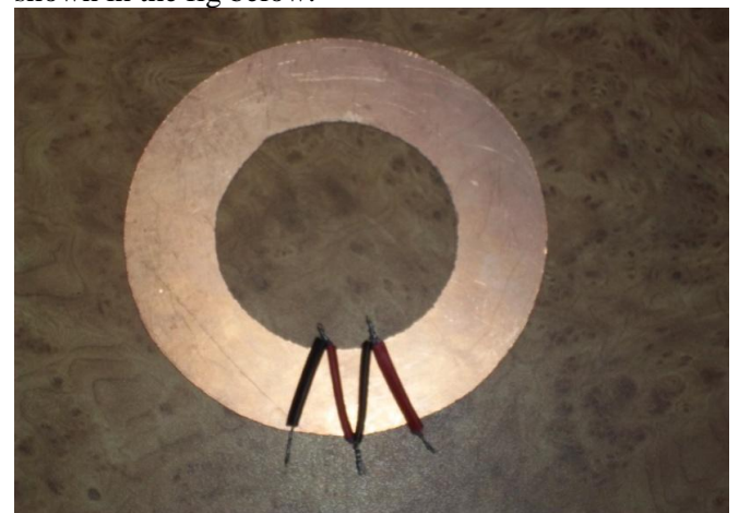
Fig 6 Thermocouples mounted on the GPB
