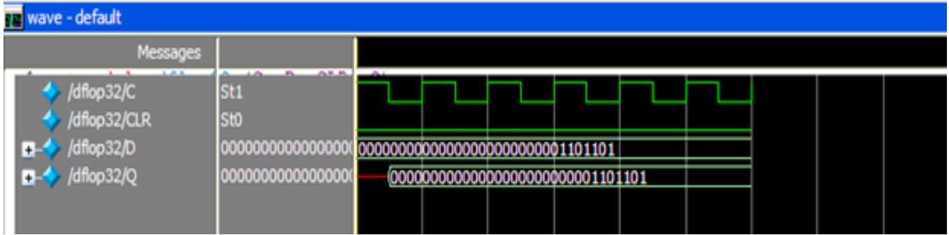
Figure 1.7: Simulation result of delay module
