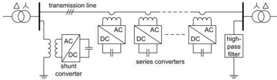
Figure 2: Complete diagram of DPFC.
