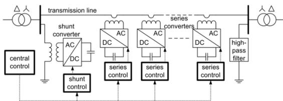
Figure 3: DPFC with series shunt and centralized controllers.
