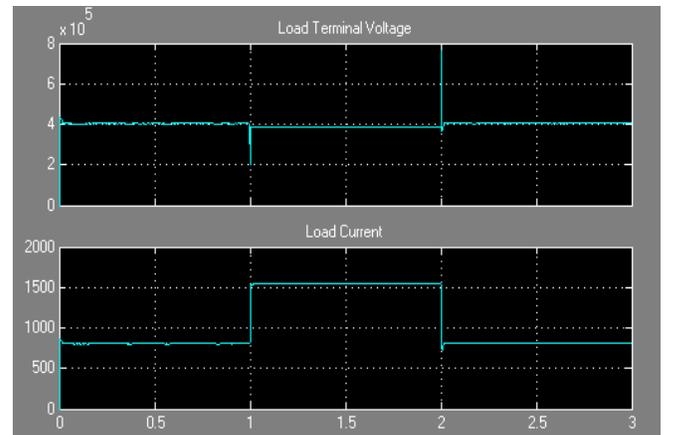
Figure 6: voltage and current at load when DPFC is turned on.
