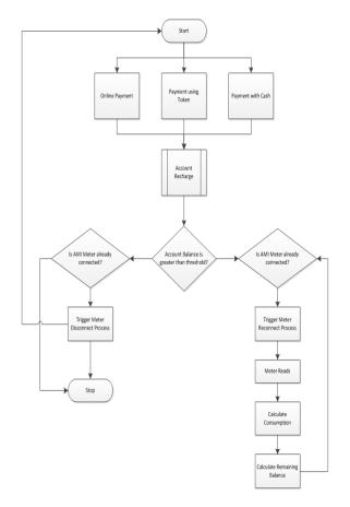
The above shown flow diagram tells us how exactly the operation is carried out, starting from the payment modes for the recharge to the checking of amount greater than threshold values which is considered as the minimum sufficient required balance to the starting of the meter operations and then carrying out with the same process again.
