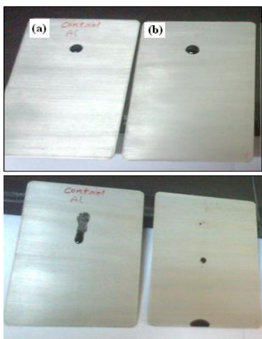
Fig. 8 Carbon black mixed with vegetable oil on Al substrate (a) Neat polyester & (b) PDMS modified polyester
