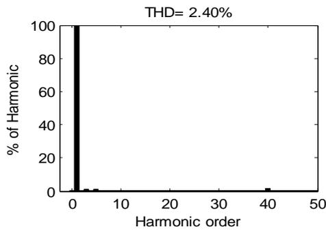
Fig. 5 Harmonic spectrum of line current ( $i_{sa}$ ) under balanced load
