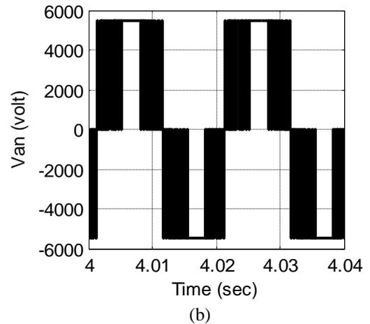
Fig. 7 (a) AC side line-to-line voltage ( $V_{ab}$ ) (b) Line-to-neutral voltage ( $V_{an}$ ) under balanced load
