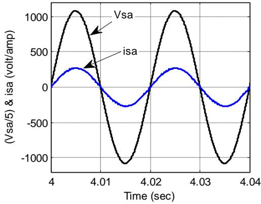
Fig. 4 Source phase voltage ( $V_{sa}$ ) and line current ( $i_{sa}$ ) under balanced load
