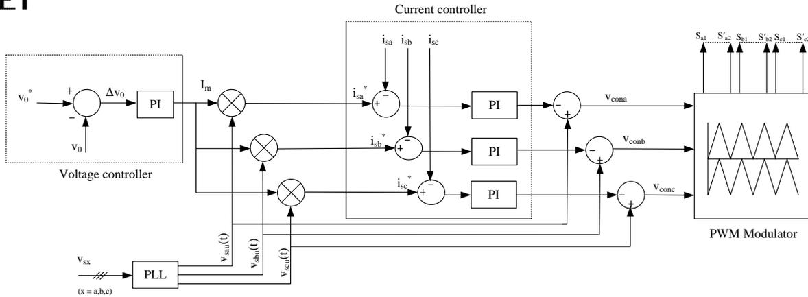
Fig.2 Schematic diagram of 3-phase, 3-level neutral point clamped multilevel rectifier control scheme.
