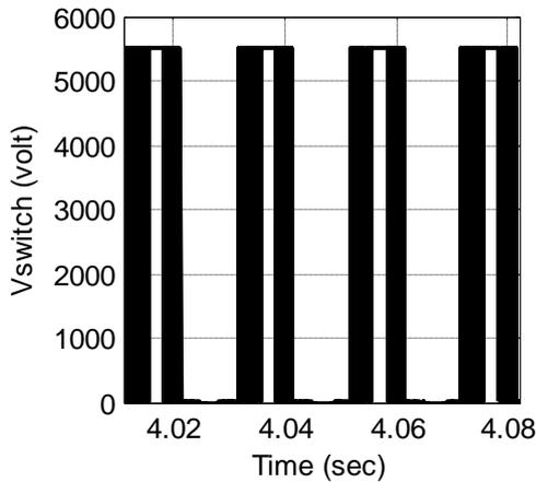
Fig. 6 Voltage across switch  $S_{a1}$  under balanced load
