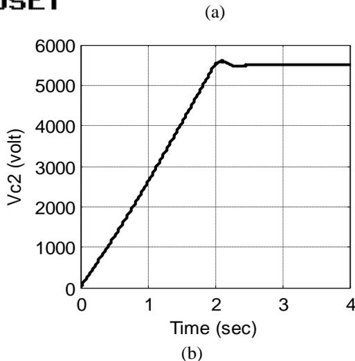
Fig. 8 (a) Voltage across dc link capacitor  $C_1$  (b) Voltage across dc link capacitor  $C_2$ , under balanced load
