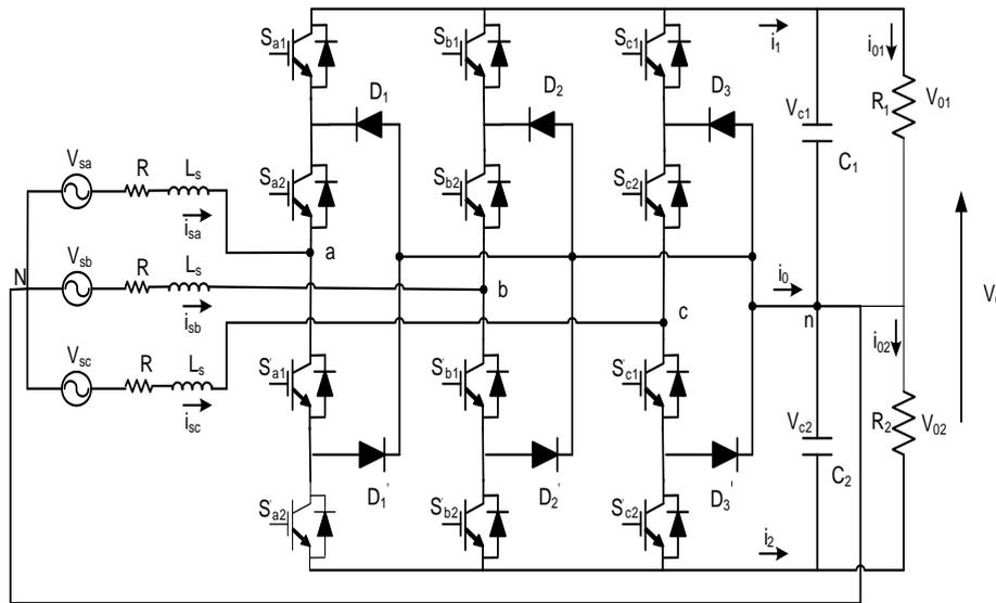
Fig.1 Three-Phase Neutral-Point Clamped Active Front End Three-Level Rectifier
