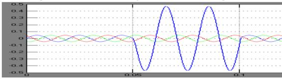
**Fig.4a: Load Current for Single Line to Ground Fault (without compensation)**
