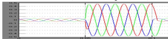
**Fig.4c: Load current for Three Fault (without compensation)**
