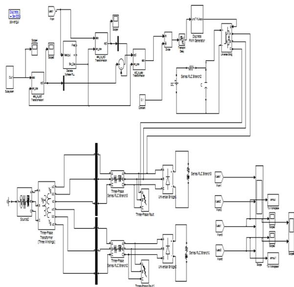
Fig.3: Simulation Diagram of Test System for DSTATCOM
