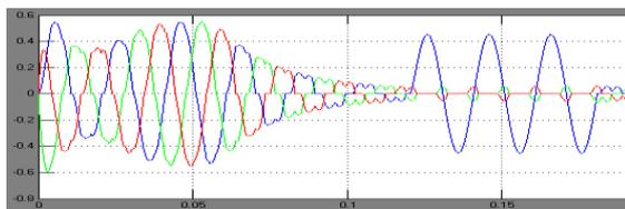
Fig.8a: Load Current for Single Line to Ground Fault (without compensation)
