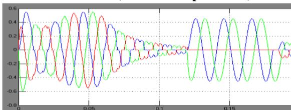
Fig.8b: Load Current for Double Line to Ground Fault (without compensation)
