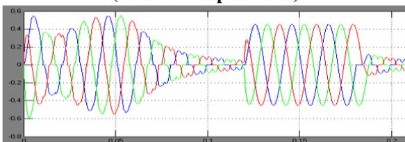
Fig.8c: Load current for Three Fault (without compensation)
