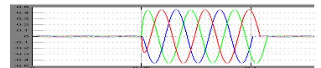
**Fig.6c: Load current for Three Fault (without compensation)**
