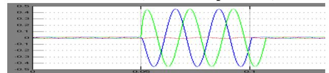
**Fig.6b: Load Current for Double Line to Ground Fault (without compensation)**
