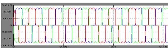
**Fig.5a: Load current (without compensation)**
