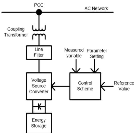
Fig.1: Schematic Representation of DSTATCOM
