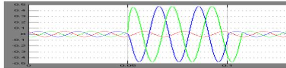
**Fig.4b: Load Current for Double Line to Ground Fault (without compensation)**
