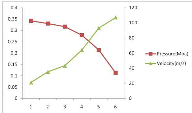
Figure 6: Pressure and Velocity relation for Isothermal & constant Exhaust mass flow
