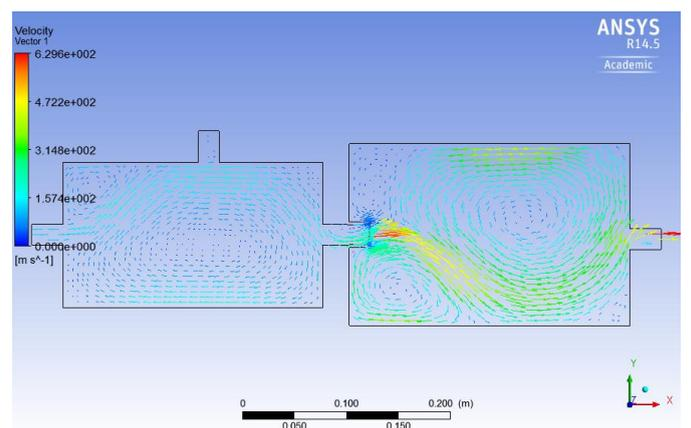
Figure 6: Velocity Vectors for mass flow rate of 3.05 kg/s Exhaust gas from the exhaust pipe and 0.0051 kg/s of air from air box
