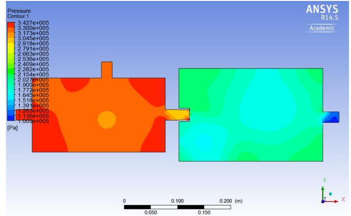
Figure 5: Pressure Contours for mass flow rate of 3.05 kg/s Exhaust gas from the exhaust pipe and 0.0051 kg/s of air from air box
