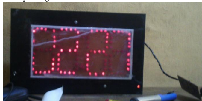
Figure 10: Final appearance of the Countdown Timer Reminder in operation displaying 02:27.
