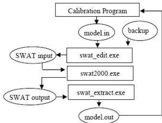
Fig 5 Interaction between a calibration program and SWAT in SWAT-cup
