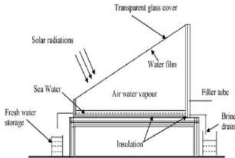
Fig 2: Passive type solar still
