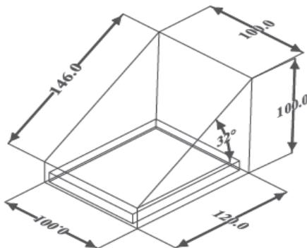
Fig 3: Single slope solar still
