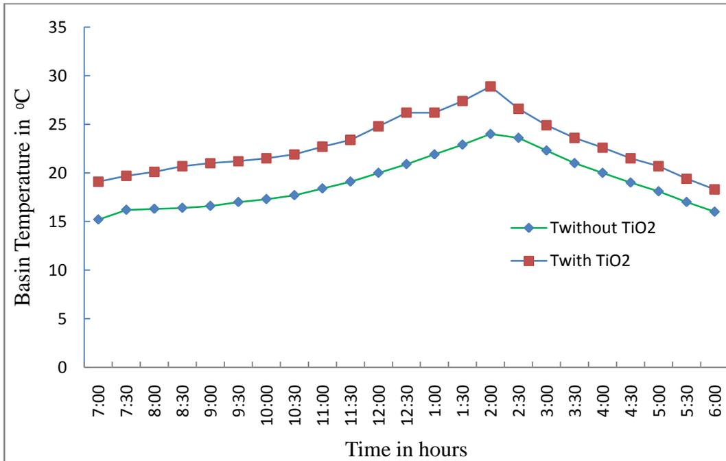
Fig 5: Variation of Basin Temperature with Time
