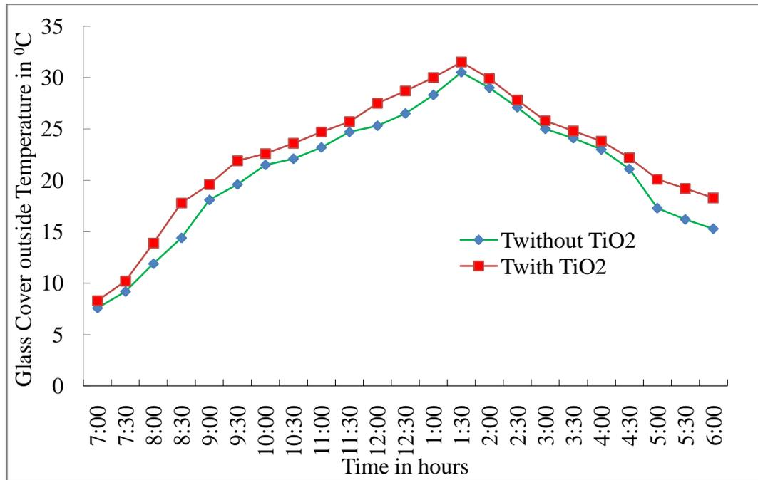
Fig 8: Variation of Glass Cover Outside Temperature with Time
