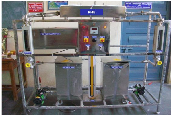
Fig.1 Experimental setup of plate heat exchange.
