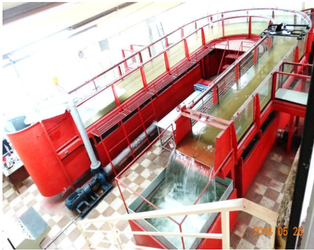
Figure (1): a view of the 180 degree sharp bend multipurpose flume located in the laboratory of advanced hydraulic structures in Persian Gulf University.
