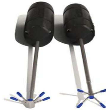
Figure (3): Two different probes of the Vectrino. On the right, the receiving beams on down looking mode, and on the left, the receiving beams on side looking mode [xiii].
