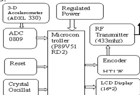
Fig 1(a) Block Diagram of Transmitter
