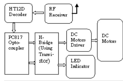
Fig 1(b) Block Diagram of Receiver
