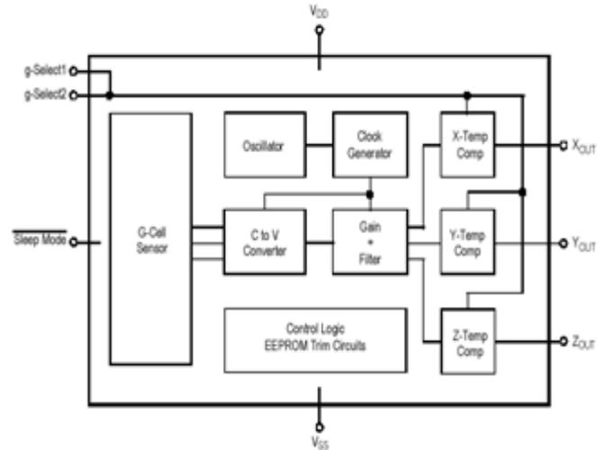
Fig 2 MEMS Accelerometer
