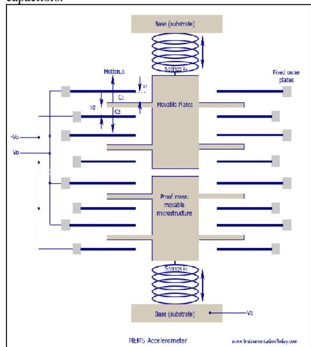
Fig 3 G-cell Accelerometer Structure
