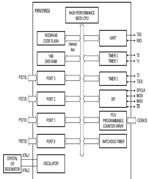
Fig 5 Microcontroller Block Diagram
