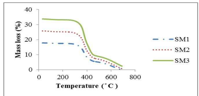
Fig 3 Effect of the Fiber Loading On Thermal Properties of Composites
