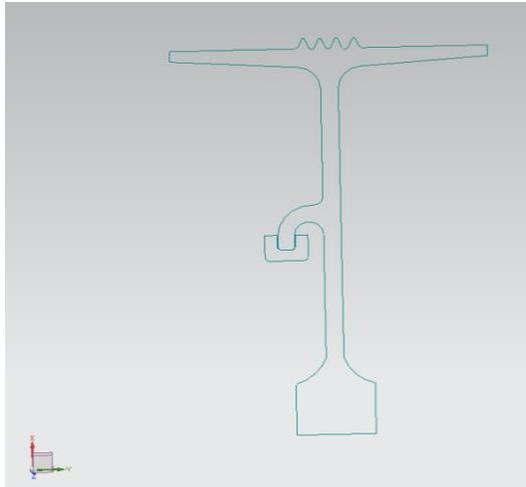
Figure 1 2D sketch seal damper model
