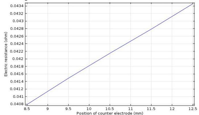
Figure 6. The plot shows the electric resistance of the pacemaker electrode in relation to the distance between the counter electrode and the working electrode.
