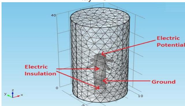
Figure 4. Boundary conditions and mesh
