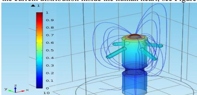
Figure 5. The plot shows the electrostatic potential distributed on the surface of the electrode. The total current density is shown as streamlines.
