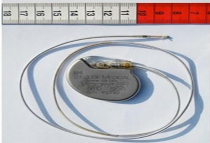
Figure 1. A puls generator of a pacemaker with electrode.
