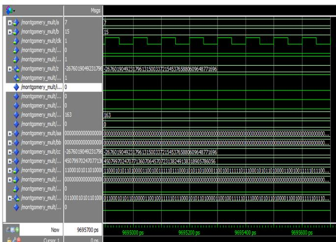
Fig 5. Generated waveform of Montgomery multiplier
