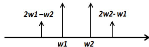
Fig 2 (a) Two input wavelengths w_1 w_2 and the arising sidebands due to FWM
