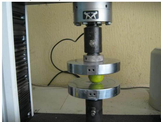
Fig. 1: Lime undergoing quasi-static compression
