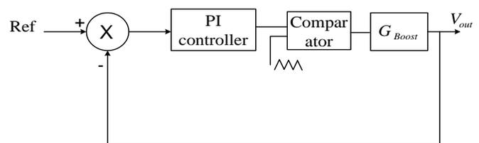
Figure 4. Control method scheme based on output voltage
