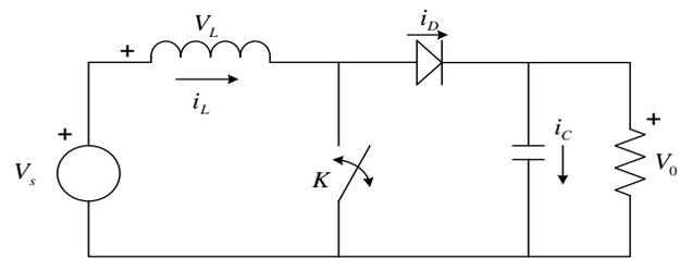
Figure 1. Topology of DC-DC Boost converter
