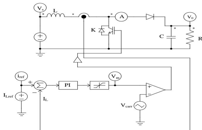
Figure 5. Control method based on inductor current
