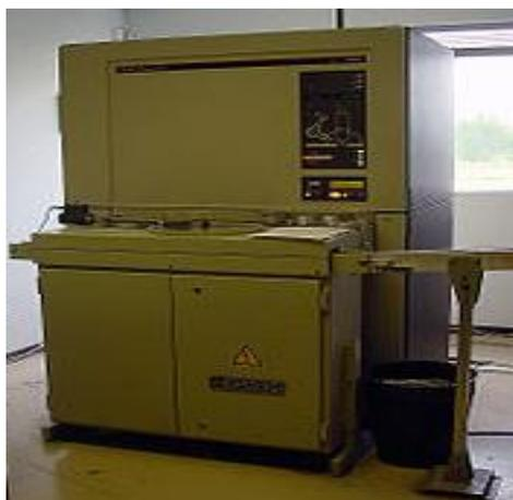
Figure 9. X-ray Fluorescence Unit
