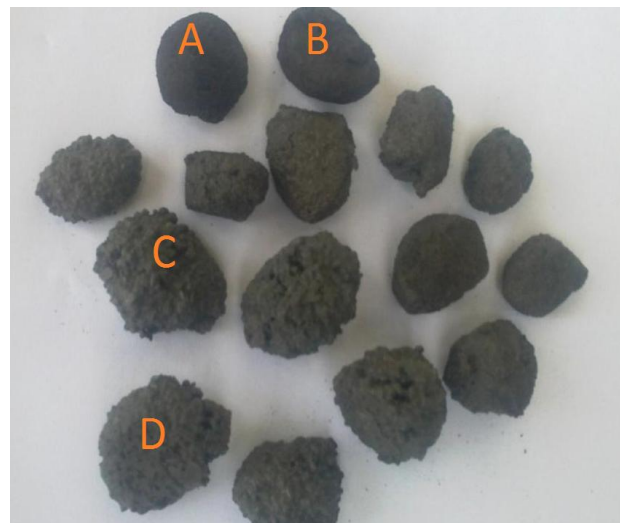
Plate 2: Agglomerates of 9-21 mm. Pellets 'A' and 'B' are fine concentrates and natural resin bonded while pellets 'C' and 'D' are coarse concentrates and cement bonded.
