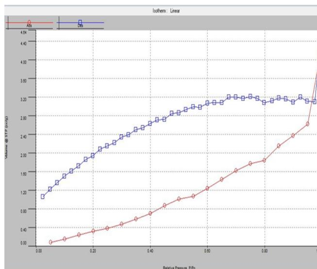
Figure 3b: BET isotherm for dowex 50W8x at 77 K
