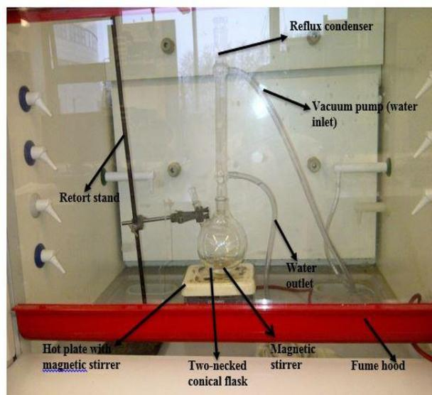
**Figure 1: Batch process Esterification process set-up.**
