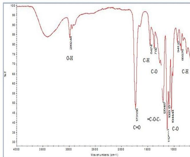
Figure 7: FTIR-ATR spectra for amberlyst 36 at 60 °C
