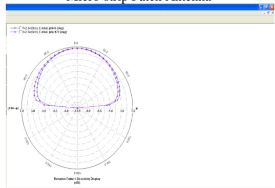
Figure (4): Radiation pattern in 2D of the Proposed E slotted Square Shape Micro-strip Patch Antenna
