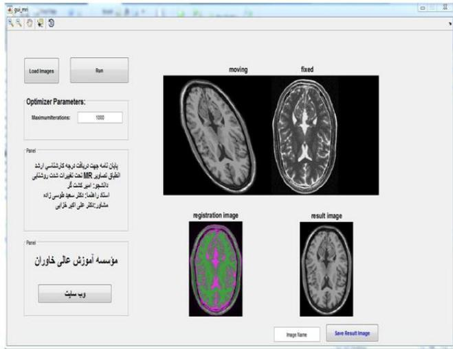
This user link consists of several parts. The first part is associated with image loading. All the formats that are supported for the matlab software can be loaded in this tool, too. In the second part the optimization parameter is adjusted. This parameter determines the maximum number of adaption operation repetition. Naturally the more this number is, the more likely the adaption will be. In figure 2-5 the view of this part has been shown.
