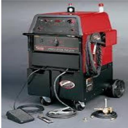
Fig 3.1 GTA welding machine.
