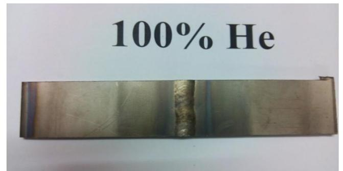
**Fig 4.5 welded job for making tensile test specimen, when 100% He used as a shielding gas.**
