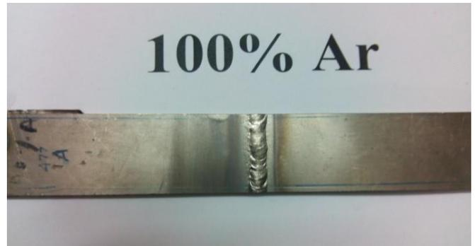
**Fig 4.4 welded job for making tensile test specimen, when 100% Ar used as a shielding gas.**
