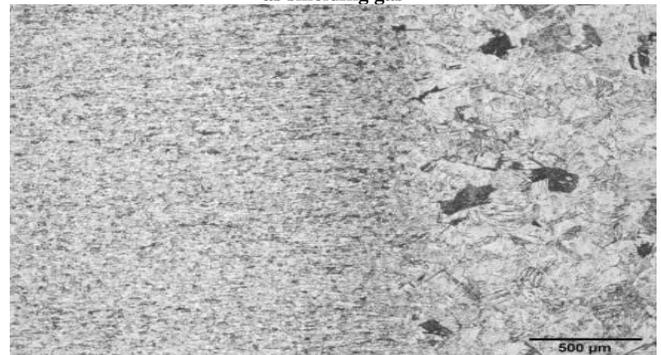
Fig 4.11 microstructure of heat affected zone (HAZ) for 100% Ar as shielding gas
