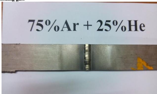
**Fig 4.3 shows welded job for making tensile test specimen, when 75% Ar + 25% He used as a shielding gas.**
