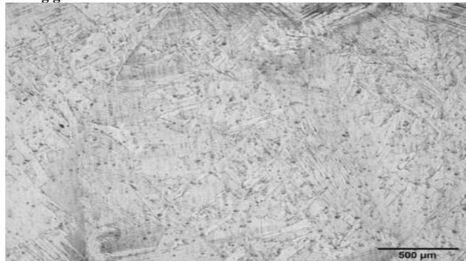
Fig 4.8 weld metal microstructure of pure titanium grade 2 with 75%Ar + 25% He as shielding gas
