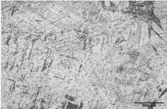
Fig 4.7 weld metal microstructure of pure titanium grade 2 with 100% Ar as shielding gas.
