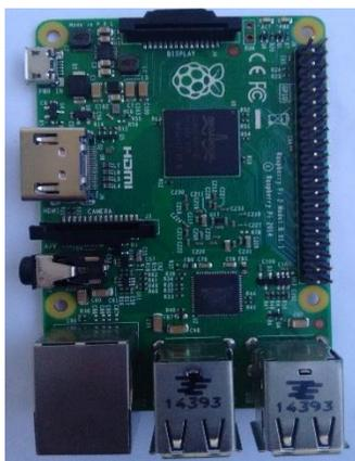
Figure 3: Raspberry Pi 2, Model B.
