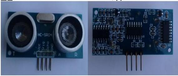
Figure 2: HC-SR04 Ultrasonic Sensor
