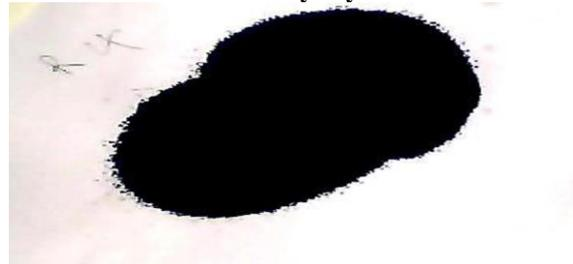
Figure 1. Bone charcoal obtained at 500°C, 90min and 2.5bar.
