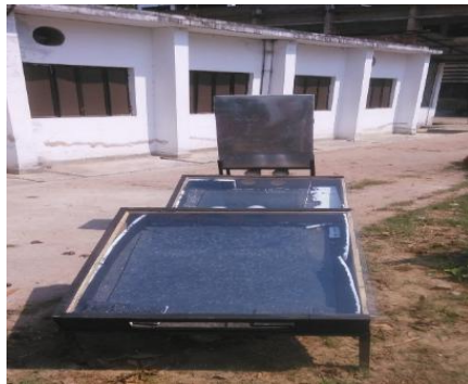
Plate: Front view of modified natural circulation solar dryer
