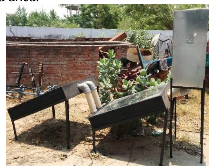
Plate: Side view of modified natural circulation solar dryer
