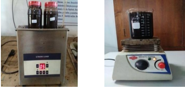
Fig.2.1 Nanofluid preparation using ultrasonicator and Magnetic stirrer
