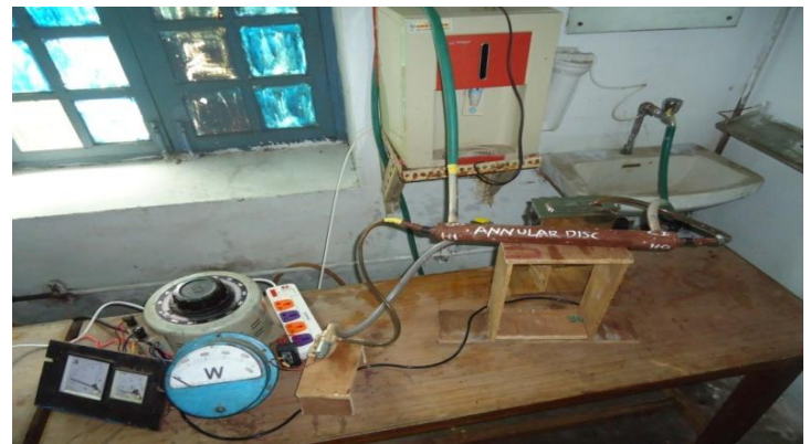
Fig.3.2 Experimental setup of heat exchangers with Annular disc
