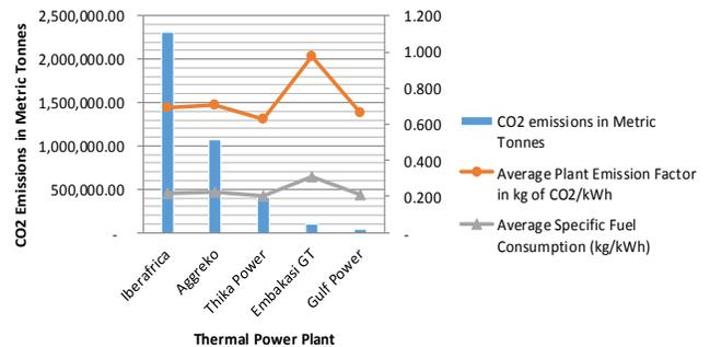
Figure 3. Comparison of Plant CO<sub>2</sub> Emission Factors and Average Specific Fuel Consumption rates
