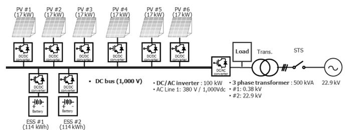
Fig. 1: Configuration of an integrated DERs in distribution system
