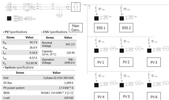
Fig. 2: Configuration of the modeled DERs in RSCAD/RTDS
