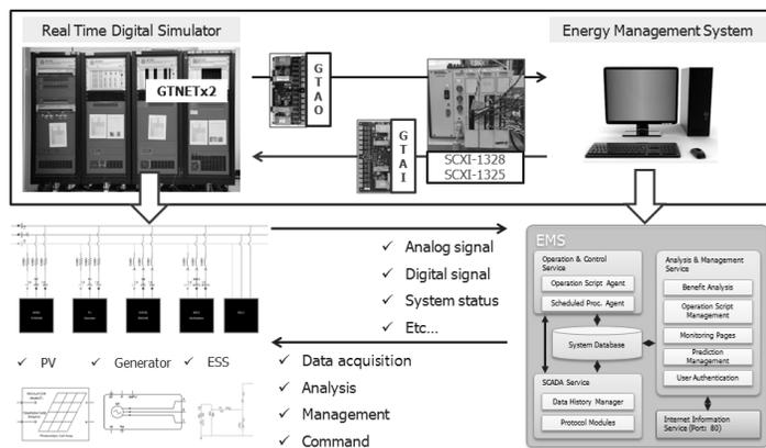
Fig. 3: Configuration of the HILS setup for optimal operation of DERs with EMS
