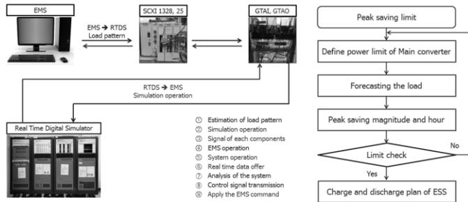
Fig. 4: HILS operation procedure with EMS (a) and optimal operation steps of EMS (b)
