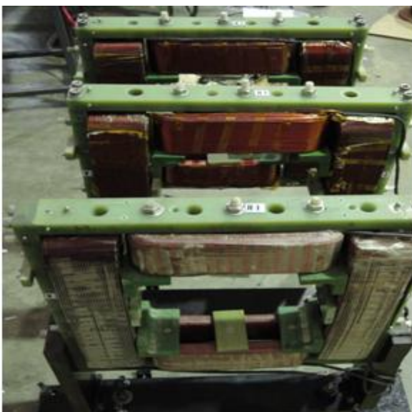
Figure 10: Fast corrector magnet assemblies for local orbit correction trails.
