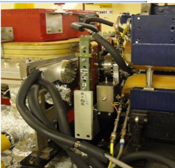
Figure 10: Fast corrector magnet assemblies for local orbit correction trails.
