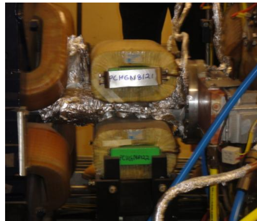
Figure 1: Combined function steel cored corrector magnet in the ring.
