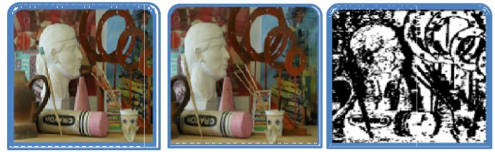
Left camera Image right camera image Disparity Map Figure:13 Horizontal Line Based Method image and Disparity Map
