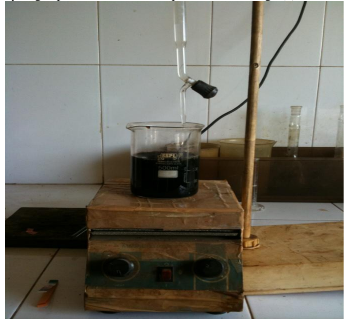
Fig. (1) Experimental set-up of fenton's process
