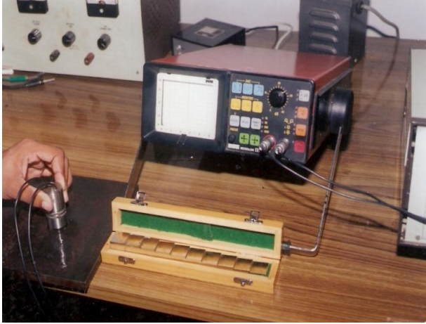
Fig 7: Experimental setup for surface roughness measurement (2)
