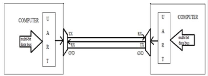
When receiving, the UART receives the data serially on the RxD pin and provides the parallel data to the application. Fig.2.
