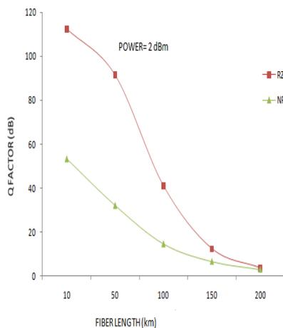
Fig 4: q factor v/s fiber length (power= 2dBm)
