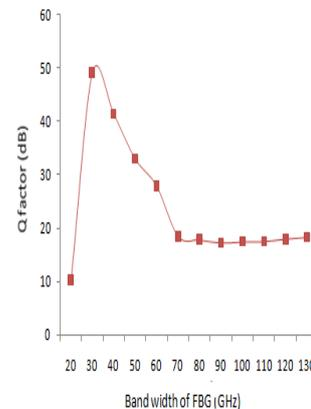
Fig 5: q factor v/s Bandwidth(GHz)
