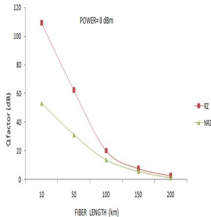
Fig 3: q factor v/s fiber length (power=0dBm)
