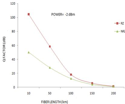
Fig 2: q factor v/s fiber length (power= -2dBm)
