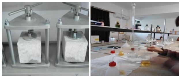
Figure 3.2.1: Images of water penetration and chloride content test
