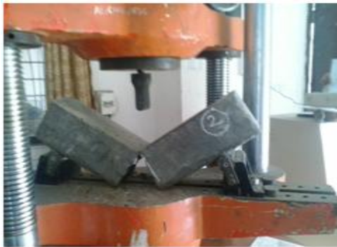
Fig.2 Test specimen of flexural test
