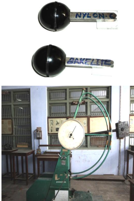
FIG. 4 IMPACT TEST OF KNOBS (A) Test specimen (B) Impact testing machine
