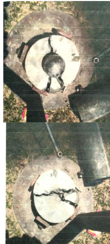
Fig. 2 Failed specimens under impact test
