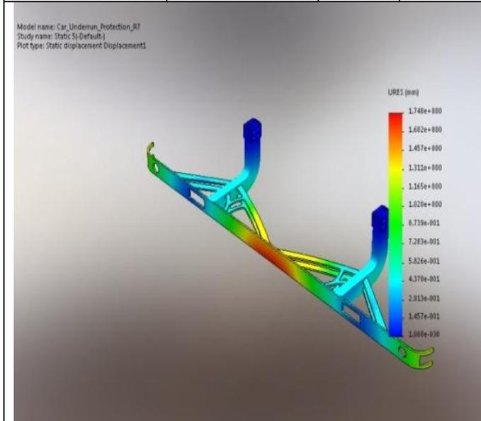
**Figure 3: Displacement 1 of P1 load**
